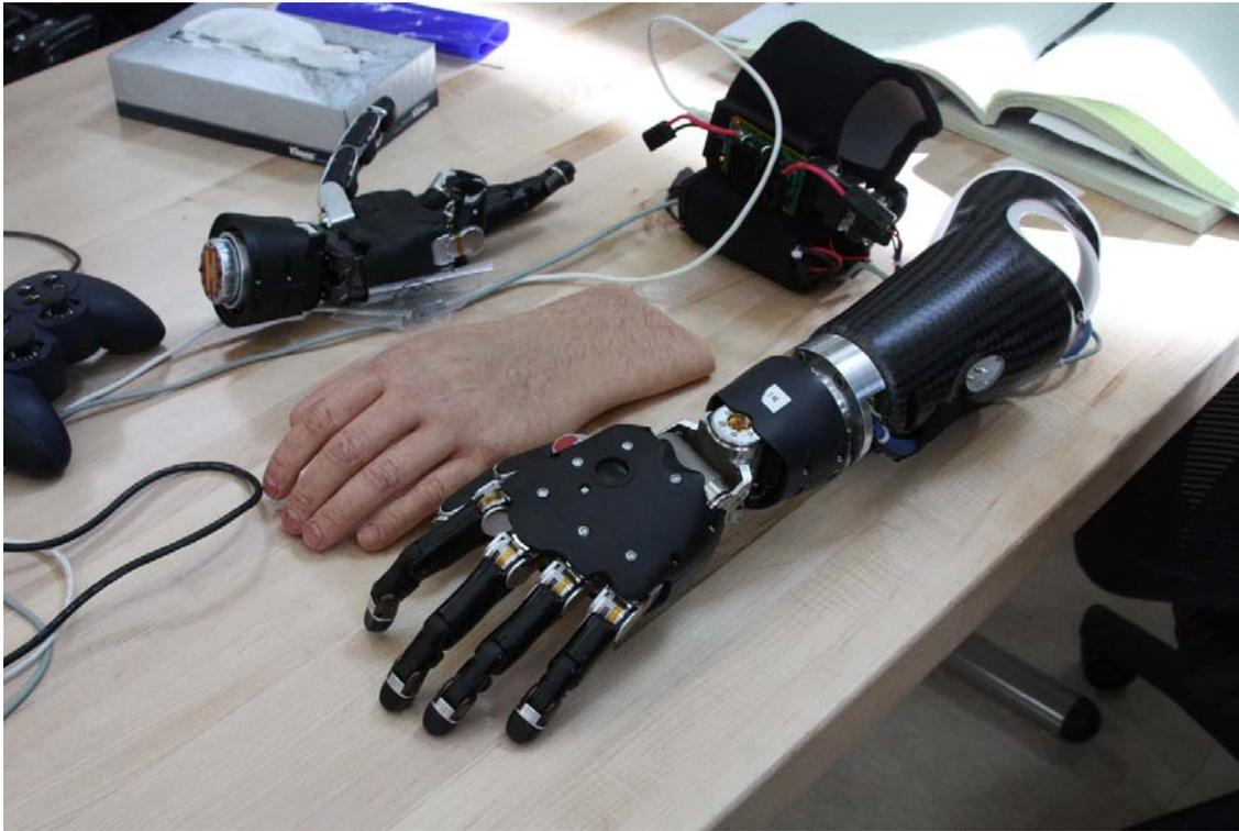
Figure 3. A Mechanical Prosthetic Hand with a Look-Alike Hand Cover.
